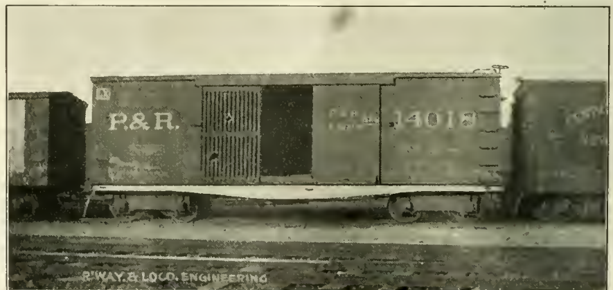
MODERN BOX CAR WITH PRESSED STEEL SIDE SILL APPROXIMATING TO ROCKERSILL SHAPE.
